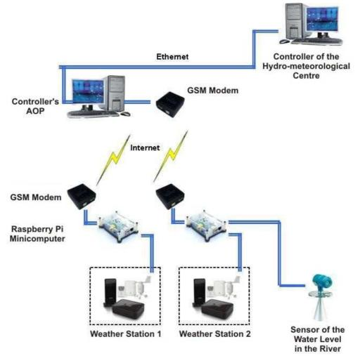
Figure 1 – Block diagram of a computer system
